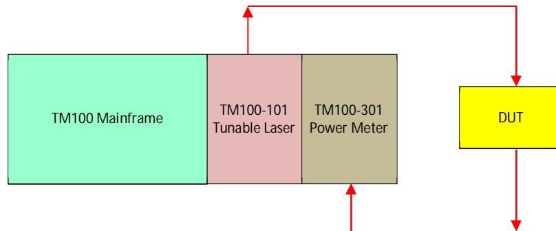
Using tunable laser and power meter to test optical component's characteristics, such as transmission or reflection spectrum, insertion loss, bandwidth, etc. Such as to test a DWDM filter.
