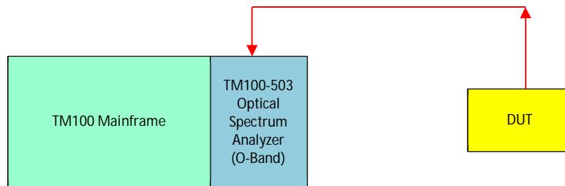
Fast scanning OSA (O-band or C-band) is an ideal instrument used in DFB laser diode (wafer level) screening test to measure the SMSR. With scanning speed as high as 50ms, it can dramatically improve the measurement cycle time and therefore the throughput.
